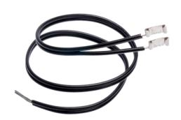
The Electrostatic Cable assembly, usually a component part of the 6500 Sonar Ranging Module, contains clips to connect between the Series 600 (or the Series 7000) Electrostatic Transducer and the 6500 Sonar Ranging Module's drive electronics. The Black (with color stripe) lead is connected to GND, and connects to the minus (-) transducer connection.
