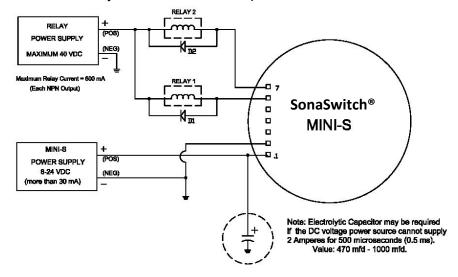
Either two separate power supplies, one for the relays and one for the SonaSwitch® MINI-S power, can be used. Or a single 12 VDC (or a 24 VDC) power supply could be used for both the Sensor and the relays (such as for using a 12 VDC, or a 24 VDC, relay).
